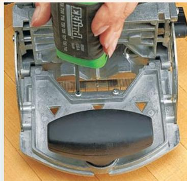
▲ **Sight Gauge.** You can adjust the horizontal sight gauge by loosening the torque screws on either side of the gauge.
