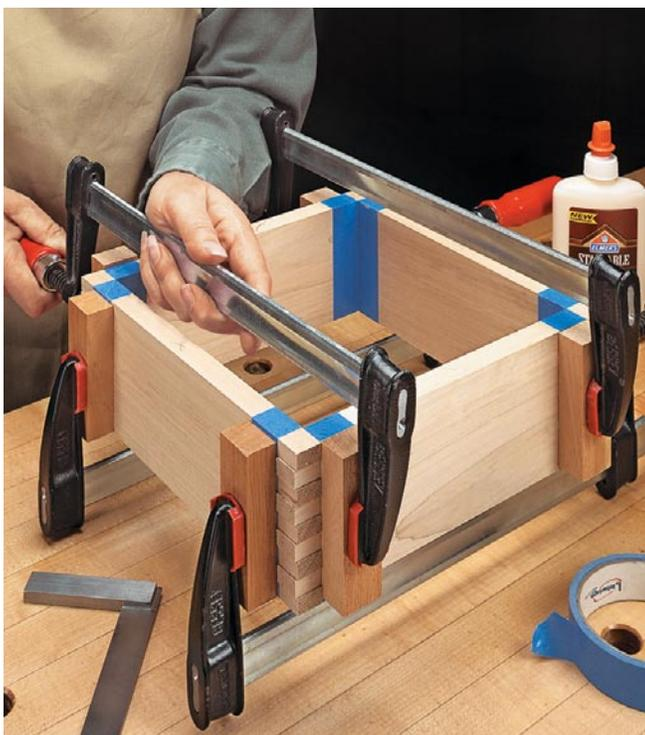
▲ **Clamping.** Position a set of blocks and clamps next to the fingers at each corner. This distributes pressure evenly and pulls the joints tight.
