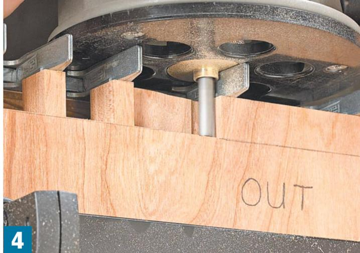
▲ **Routing the Pins.** To rout the pins, flip the finger assembly around and set the cutting depth of the straight bit. Rout the pin board with the outside face facing out.
