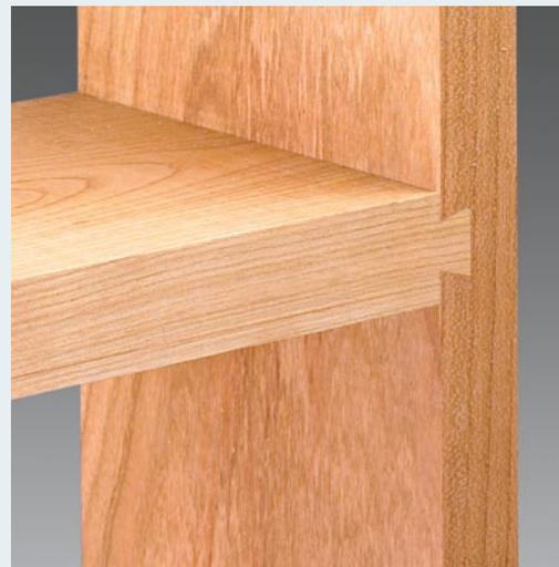
▲ **Sliding Dovetails.** The sliding dovetail shown above is the perfect way to join shelves and partitions together securely in any project.
