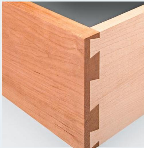
▲ **Half-Blind Dovetails.** Building drawers with half-blind dovetails is a snap — even with the variable size and spacing shown above.
