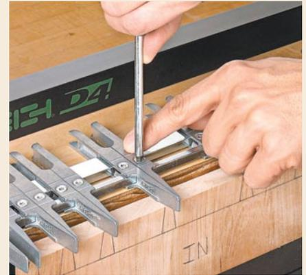
▲ **Fingers.** The adjustable half fingers allow for variable spacing and sizing of both the pins and tails of a dovetail joint to suit your project design.
