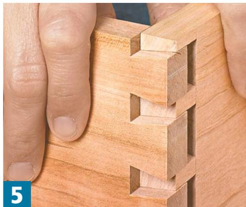
◀ **Test the Fit.** The goal is to adjust the finger assembly to rout the pins so they just slide into the tail board with firm pressure. Once you're there, you can rout all the pin boards.
