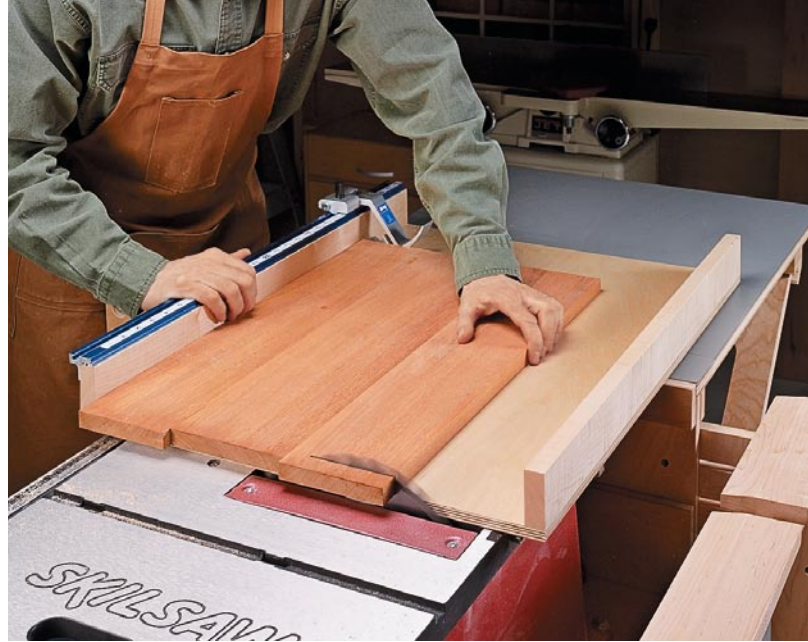
▲ Crosscut Sled. The sled lets you make accurate cuts on panels up to 20" wide. A T-track on the top lets you add a stop for cutting identical parts.
