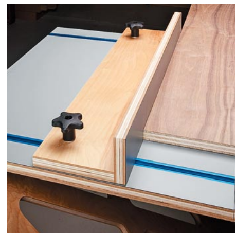
▲ Auxiliary Rip Fence. This fence rides in a pair of T-tracks in the right wing. It lets you rip wider pieces of plywood.
