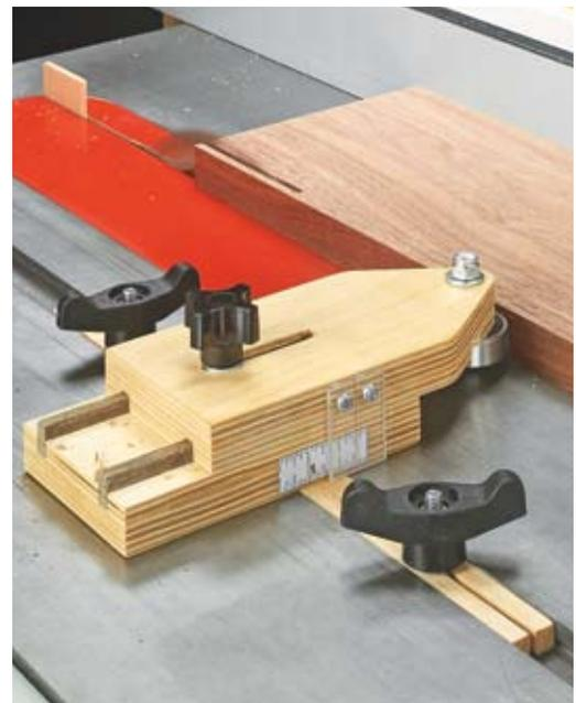
▲ **Ripping a Long, Thin Strip.** Position the jig in front of the blade and tighten it in place. The bearing gauges the workpiece thickness.
