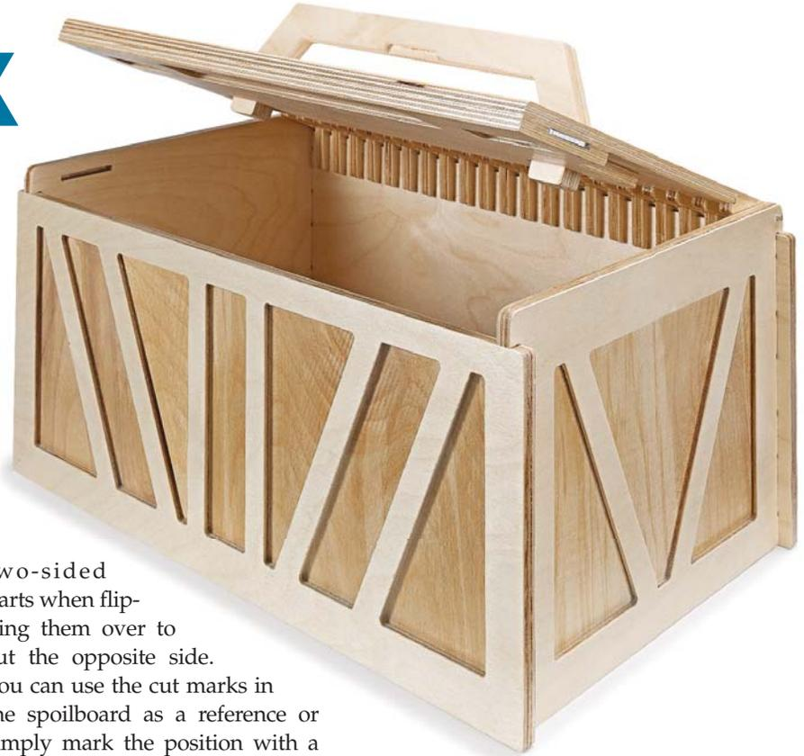
■ This toolbox is designed from the ground up to be cut with a CNC router. The sides and bottom have tabs on their edges to fit into blind mortises in the front, back, and sides. The back and top have a series of recesses on the inside for the individual pieces that form the knuckles of the hinge. The latches and handle assembly are integrated into the top. The top is also engraved with the *ShopNotes* logo. And to finish it off, decorative pocket cuts were made on the outside of the toolbox.
