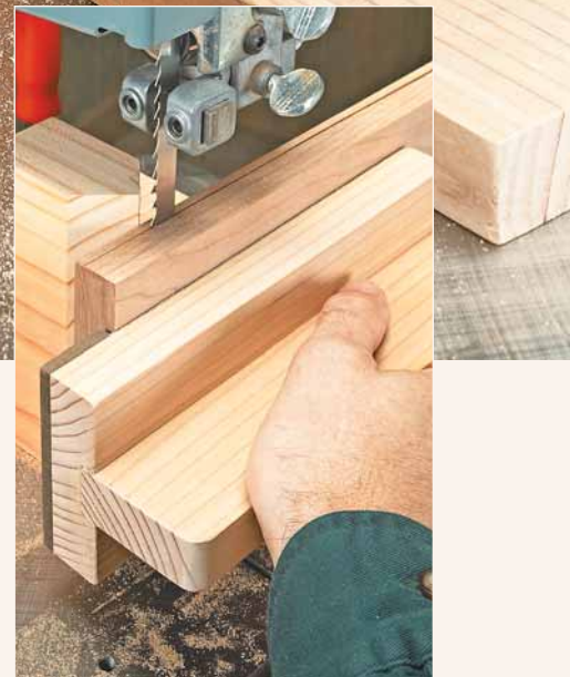
▲ Complete Control. A shop-made push block allows you to safely feed the workpiece through the end of the cut.
