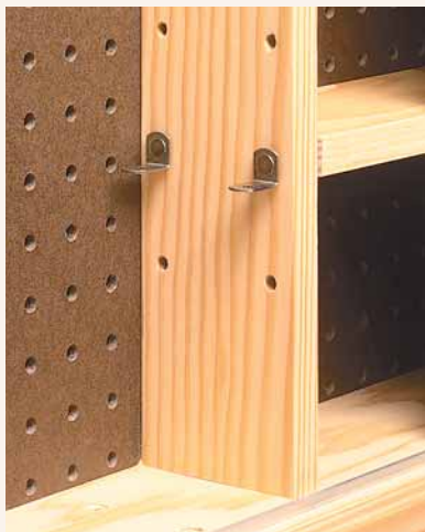
▲ Shelf Supports. Removable shelf supports are used to support the adjustable shelves inside the pegboard storage cabinet.
